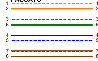
Schema collegamenti (T568B)
