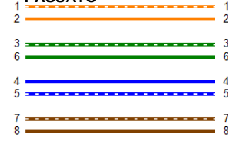
Schema collegamenti (T568B)
