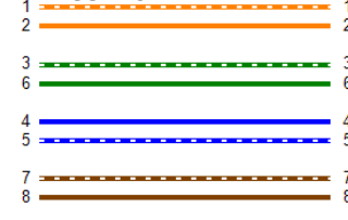
Schema collegamenti (T568B)
