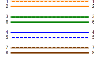
Schema collegamenti (T568B)
