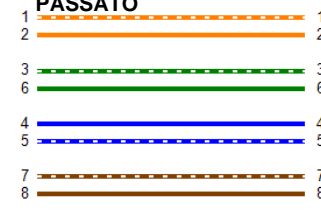
Schema collegamenti (T568B)
