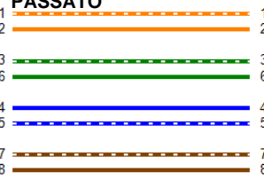
Schema collegamenti (T568B)
