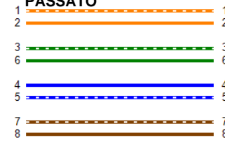
Schema collegamenti (T568B)
