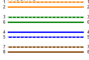
Schema collegamenti (T568B)
